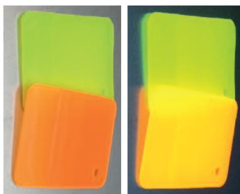
TPU sample plates with fluorescent pigments under daylight conditions
