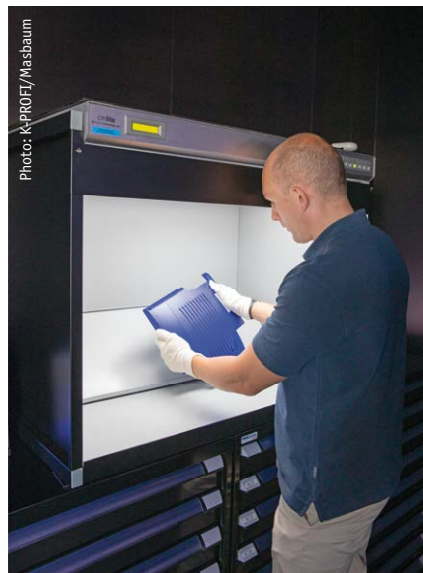
In color assessment cabins located in the darkroom, the colorist determines the color under standard light conditions.
