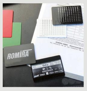
Glass fibers and glass beads normally have no effect on the marking contrast. Mineral fillers such as talcum, however, may have a slightly negative effect. What's more, the flame retardants used in certain fire-resistant products can hamper laser marking because they prevent the combustion process.
