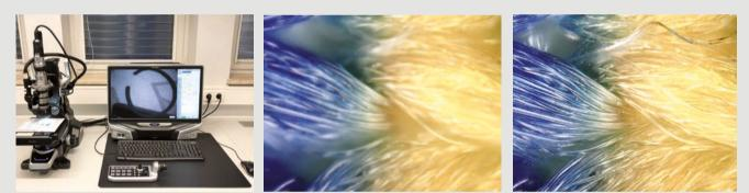
Digital microscope with computer, software and control panel
