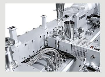
ROWA Masterbatch further optimizes efficiency, quality stability and service with its investment in the new laboratory machine ZSK 26. The twin-screw extruder from Coperion can produce the same product as its big brother ZSK 45 - but to a lesser extent. Thanks to the
